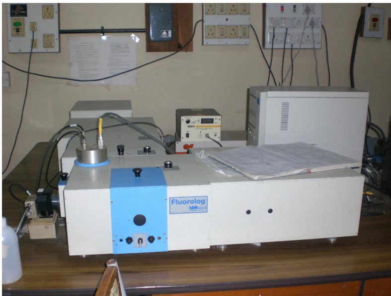
TAU fully automated fluorescence life time measurement system:
